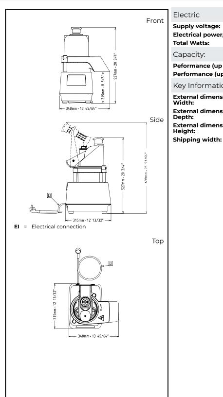
Electric Supply voltage: 115 V/1N ph/60 Hz Electrical power, max: 1kW **Total Watts:** 1kW Capacity: Peformance (up to) 330,6 lbs/cycle Performance (up to): 150 kg/hour Key Information: External dimensions, Width: 13 11/16" (348 mm) External dimensions, 12 3/8" (315 mm) Depth: External dimensions, 20 3/4" (527 mm) Height:
